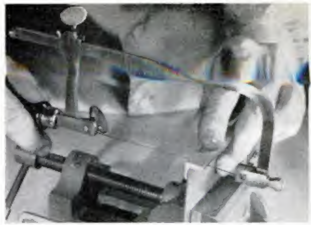
TO PREVENT BLADE WANDER , cut groove on underside, hold piece so groove is at cut starting point
